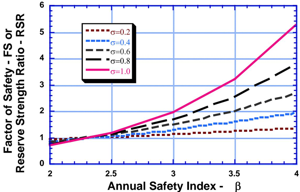
**Figure 1- Element factor of safety or system Reserve Strength Ratio as function of total uncertainties in maximum loadings and capacities and biases of unity**
