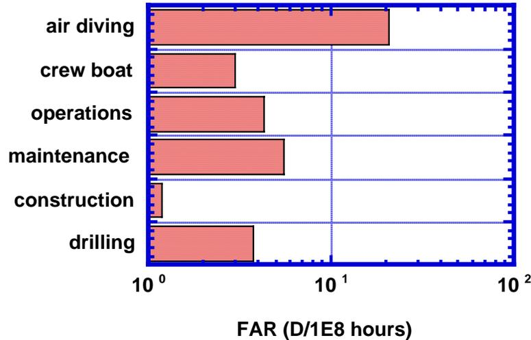
**Figure 7 – UK offshore operations mean FAR 1991 - 1996**
