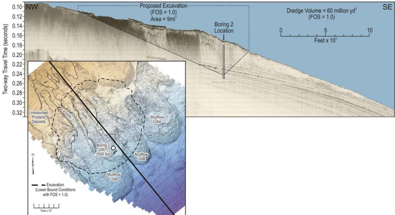
Figure 6. Superimposed on the NW-SE oriented high resolution seismic profile is the projected excavation feature centered at the well bay and extending upslope through mudflow lobes, gullies, and relatively undisturbed “slabs” of delta-front sediment. The inset image generated from multibeam bathymetry data shows the position of the seismic line with respect to geologic features of the project area. The general outline of the excavation (FOS = 1.0) is superimposed on the image.
